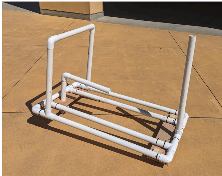
Figure 3: Full Assembled PVC Pipe Cart
