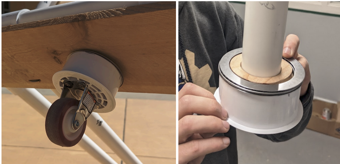
Figure 4: Detailed pictures of tiller mechanism separate (right) and in-place (left)
