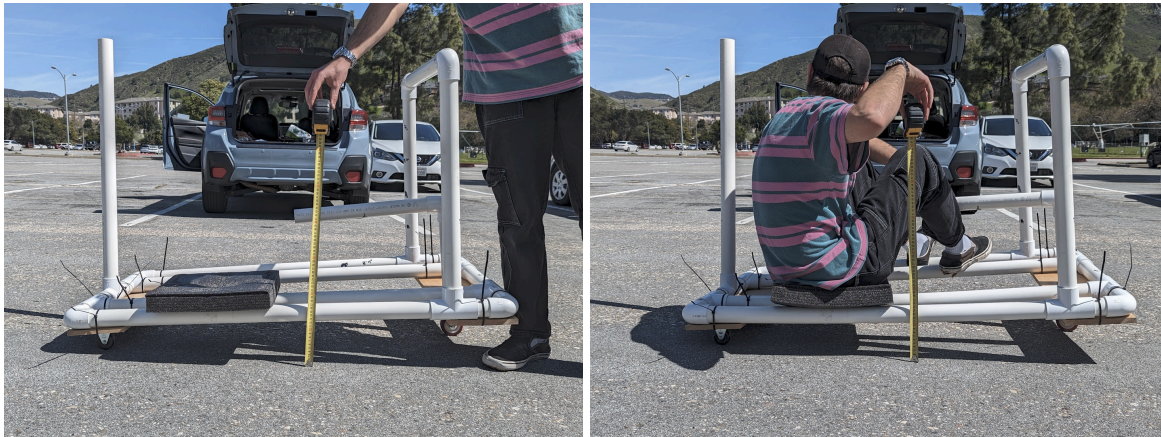
Figure 4. Deflection measurement setup with 140lb rider
